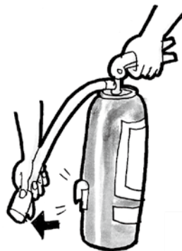
2. Unfasten the fire hose and aim its nozzle at the fire.
