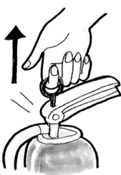
1. Pull off safety pin in upward motion.
