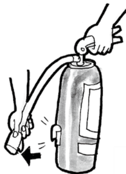
2. Unfasten the fire hose and aim its nozzle at the fire.
