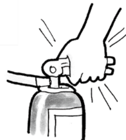
3. Clutch the lever to release the chemicals.
